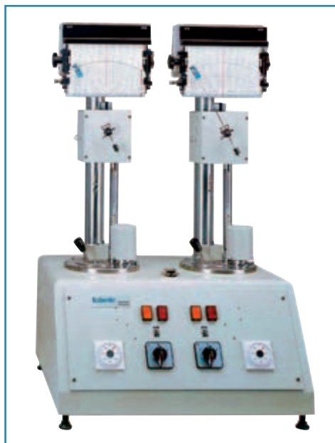
Fig. 52: Oven Rise Recorder for measuring the increase in the volume of dough pieces during the baking process (source: Brabender OHG)
