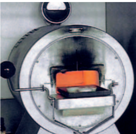
Fig. 39: Muffle furnace for ashing flour, with porcelain crucibles (source: University of Hanover)
