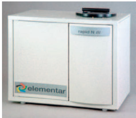
Fig. 43: Device for automatically determining the protein content by the Dumas combustion method (source: Elementar Analysensysteme GmbH)
