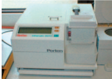
Fig. 38: Determining the moisture content of whole kernels (left) and flour (right) using near-infrared transmission technology (NIT) or near-infrared reflection spectroscopy (NIR) (sources: Brabender OHG / Mühlenchemie GmbH)
